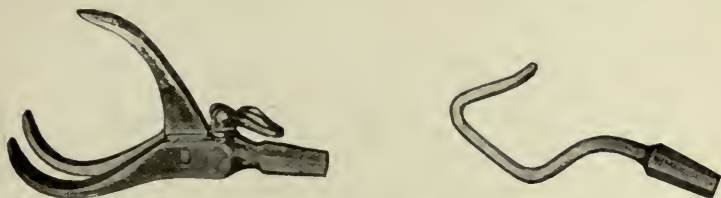
FIG. 145.—Clamp and hook serviceable for the amputated workman. The clamp serves to hold a file, brush, small hammer, etc. The hook can be used to carry a pail or to lift heavy objects.
