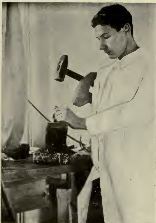
FIG. 170.—The one-armed bracemaker's apprentice already pictured in Fig. 169. This illustration shows his method of gripping the hammer between the stump, upper arm and chest.
