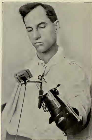
FIG. 148.—Judge Corley's apparatus for helping the man who has lost both hands to button his own collar.
