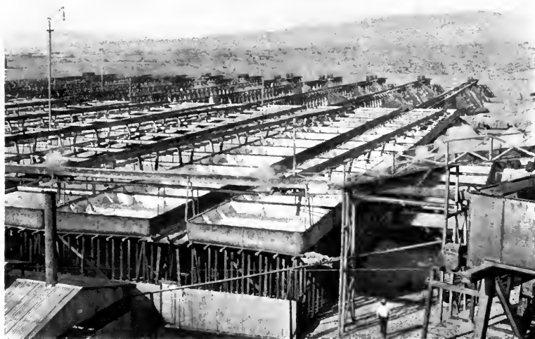
Nitrate vats at an "oficina" in the north of Chile. From nitrates comes most of Chile's income.
