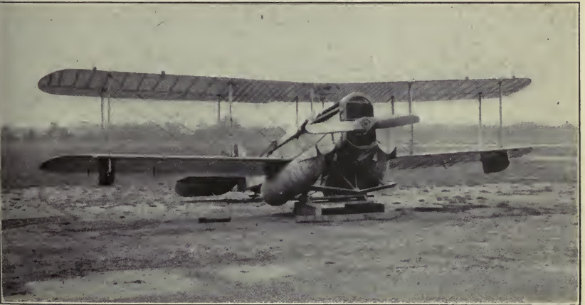
Airplane Equipped with Air Bags for Floating on the Water
