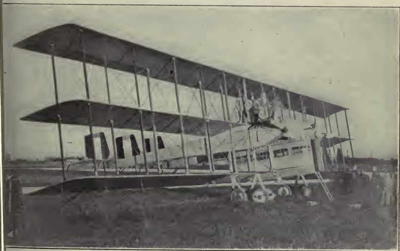
Italian Caproni Passenger Airplane. Carries About Fifteen Passengers and can be Rapidly Converted into a Bombardment Airplane
