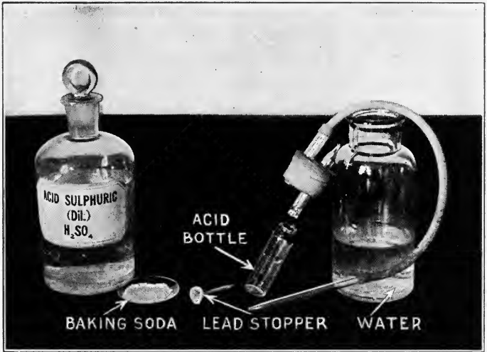
A LABORATORY MODEL FIRE EXTINGUISHER Give the use of each article and substance.
