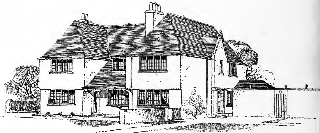
THE HON. LORD PEARSON'S COTTAGE AT COLINTON. MATERIALS: STONE WALLS AND ROUGH-CAST, WITH TILED ROOF
