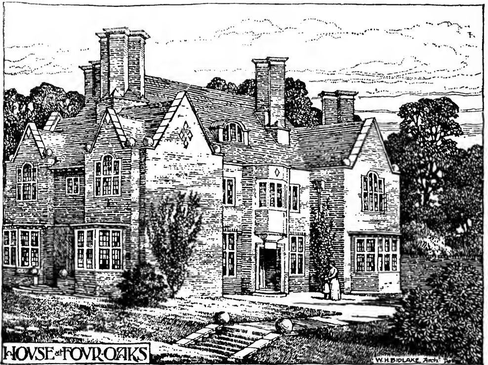
HOUSE AT FOUR OAKS, NEAR BIRMINGHAM. BUILT OF RED SANDSTOCK BRICKS, THE ROOFING OF RED TILES
