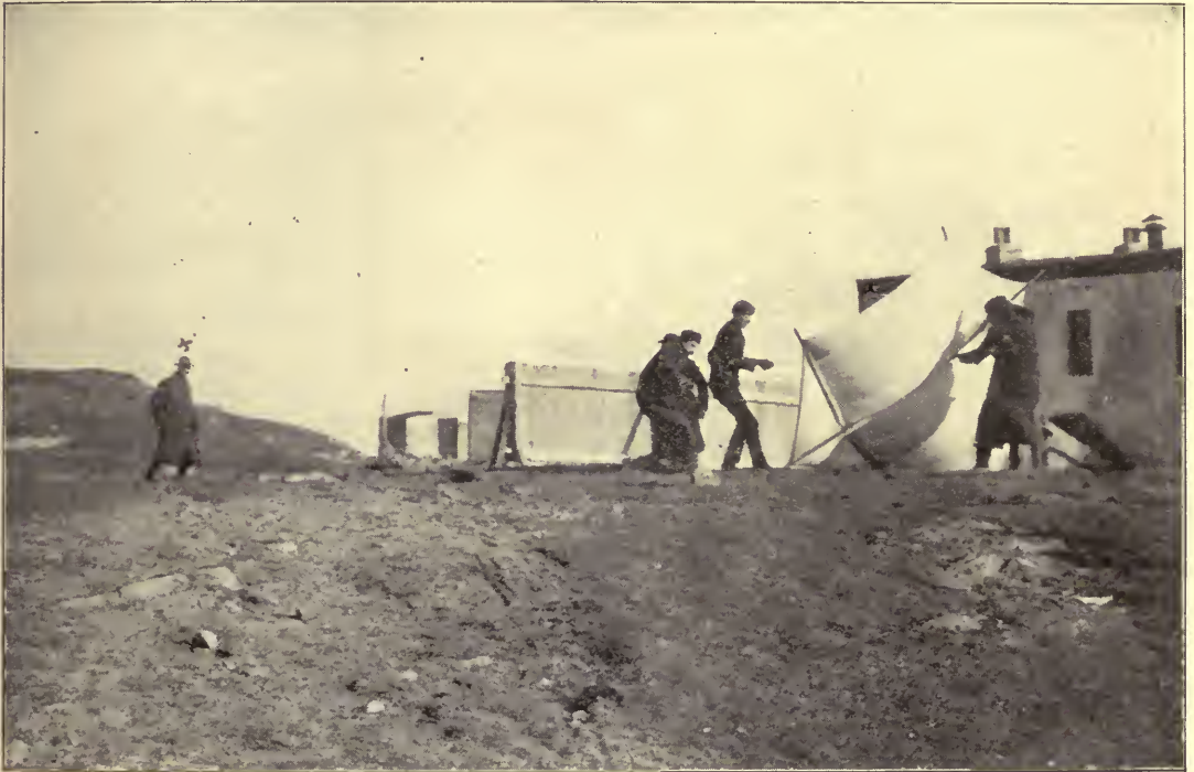
MARCONI'S ASSISTANTS PREPARING TO RAISE THE KITE WHICH SUPPORTED THE RECEIVING WIRE.
