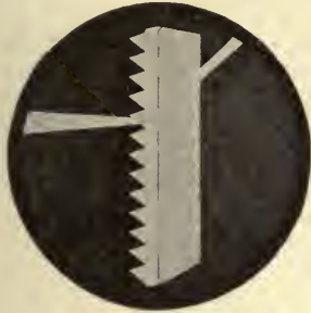
HOW THE PRISM ACTS. Showing ray of light from above, deflected to a horizontal course as it passes through the glass.
