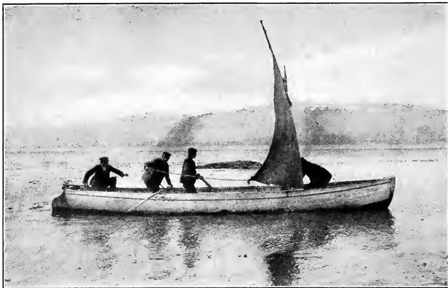
THE BOAT IN WHICH MR. FURLONG CRUISED THROUGH BEAGLE CHANNEL. ITS GREAT LENGTH AND NARROW BEAM UNFITTED IT FOR ROUGH SEA.
