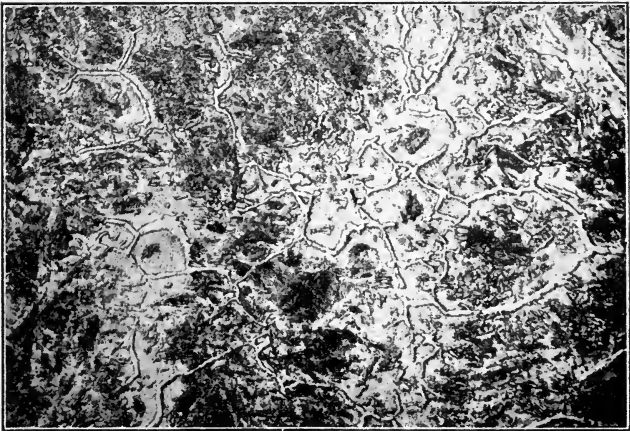
FIG. 224.—Cementite (white) forming network around Pearlite grains in 1.75 per cent Carbon Blister Steel. Magnified 15 diameters.
