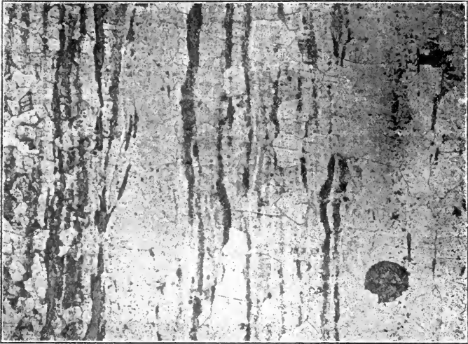
FIG. 242.—Slag in Wrought Iron, showing black in Ferrite ground mass. Magnified 60 diameters.
