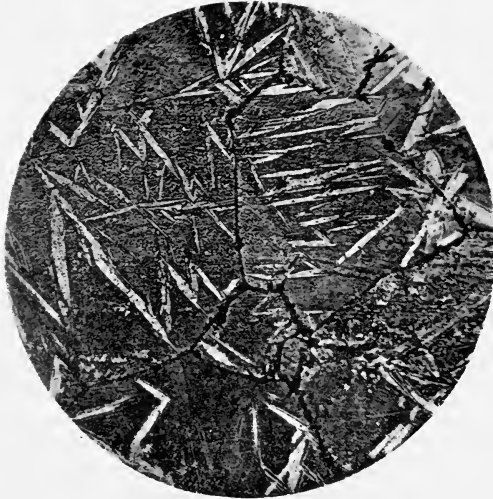
FIG. 251.—Austenite and Hardenite Structure of completely Solid Steel (C. = 1.76 per cent) quenched in water at 1,120 deg. Cen. (Gutowsky.) Magnified 200 diameters.
