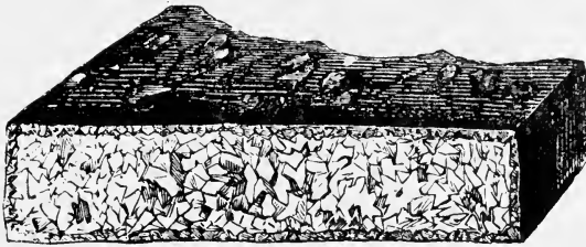
Fracture of Blister Steel.—Spring Heat.
