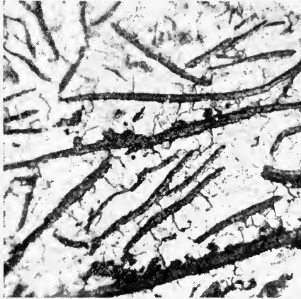
FIG. 219.—No. 1 Hematite Pig (Stead). Magnified 40 diameters. (The dark areas are graphite, the ground mass is silicon-ferrite.)
