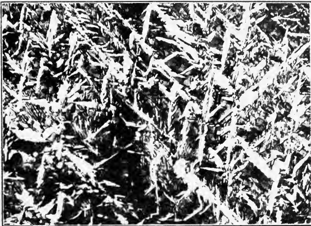
FIG. 228.—Austenite (dark) associated with Hardenite (white needles) in 1.6 per cent Carbon Steel, quenched from 1,100 deg. Cen. in iced brine. Magnified 300 diameters.
