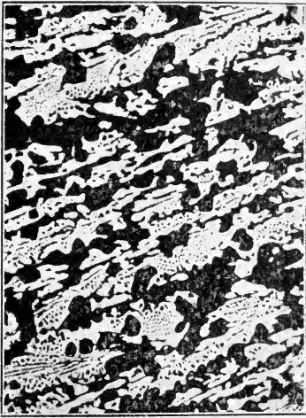
FIG. 245.—Chilled Grey Iron (Edge). White—Cementite, Black—Sorbite, Eutectic—Austenite—Cementite. V. 90 X.
