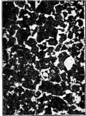
FIG. 259.—Annealed Structure of .46 per cent Carbon Steel (Ferrite and Pearlite). V. 90 X.
