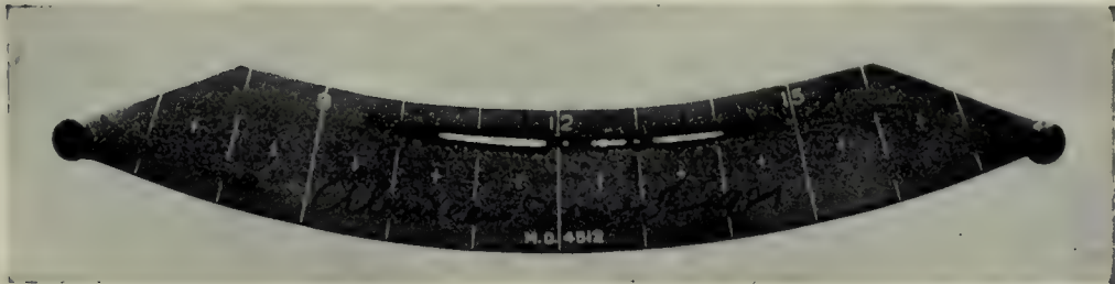
PHOTOGRAPH COPY OF A SUNSHINE RECORD
