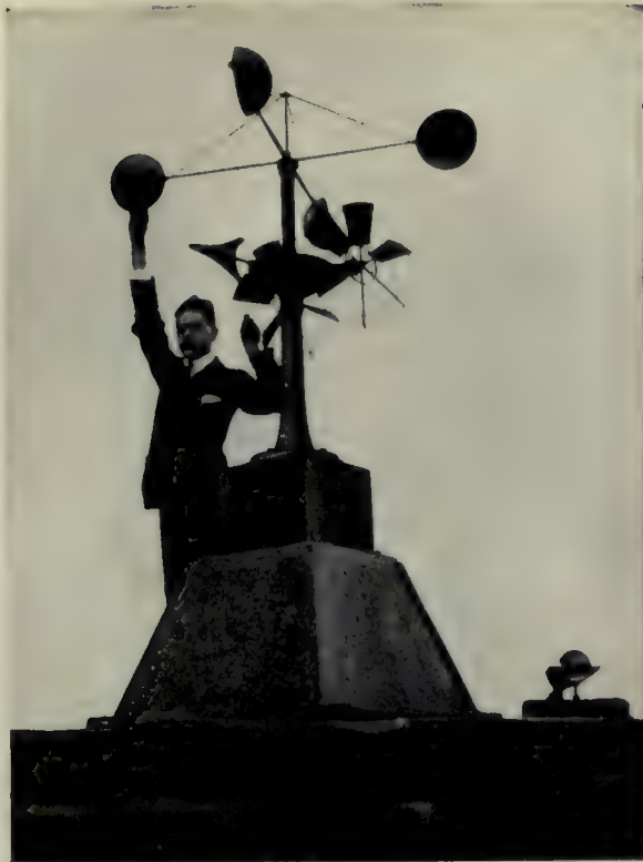
THE ROBINSON ANEMOMETER
