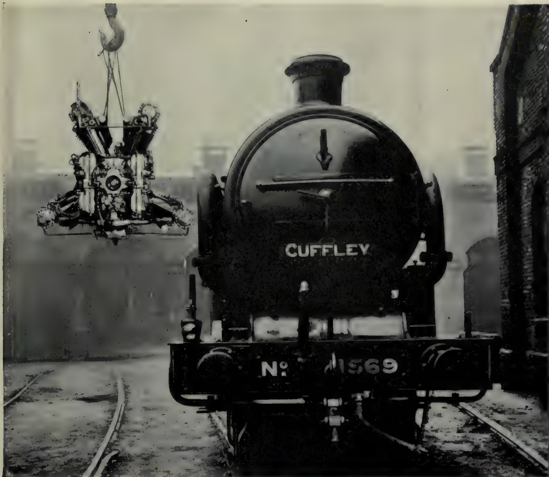
A COMPARISON IN SIZES SHOWING THE 1,000 H.P. NAPIER "CUB" AERO ENGINE WHICH WEIGHS ABOUT 1,700 LB., AND A 1,000 H.P. LOCOMOTIVE WEIGHING SEVERAL TONS
