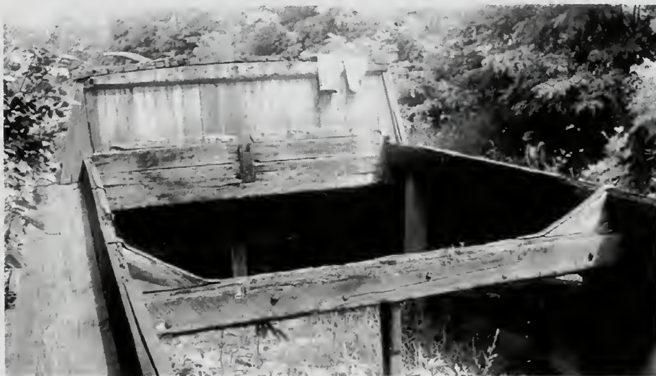
Photograph 58: Looking aft from Hay House, amidships, over cargo hold to cabins; cross brace in foreground. Diagonal brace below at right.
