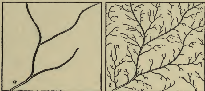
FIG. 10.—Showing the diverse action of rain on wooded and cleared fields. a , wooded area; b , tilled ground.
