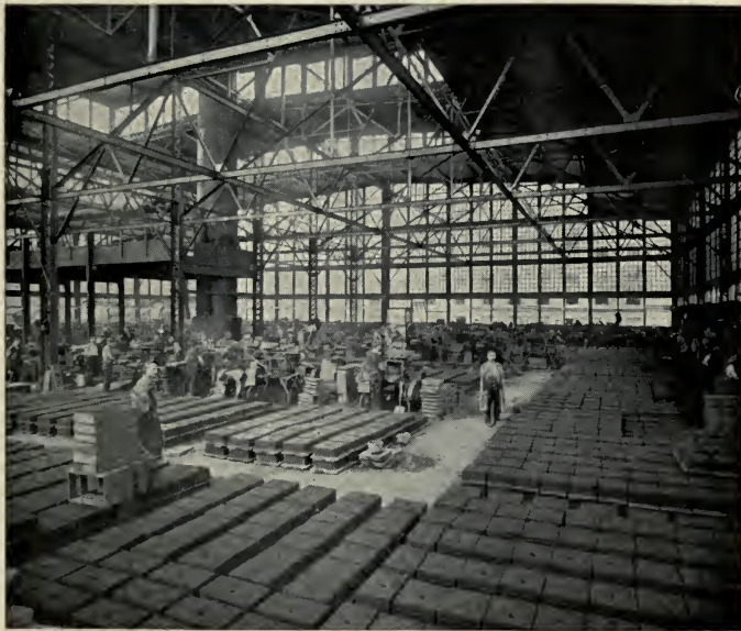
Plate XIII: Glass and steel are the principal building materials which make up this light, well ventilated foundry of the Michigan Stove Company. The air is clear fifteen minutes after a heat is off (See chapter XIII)
