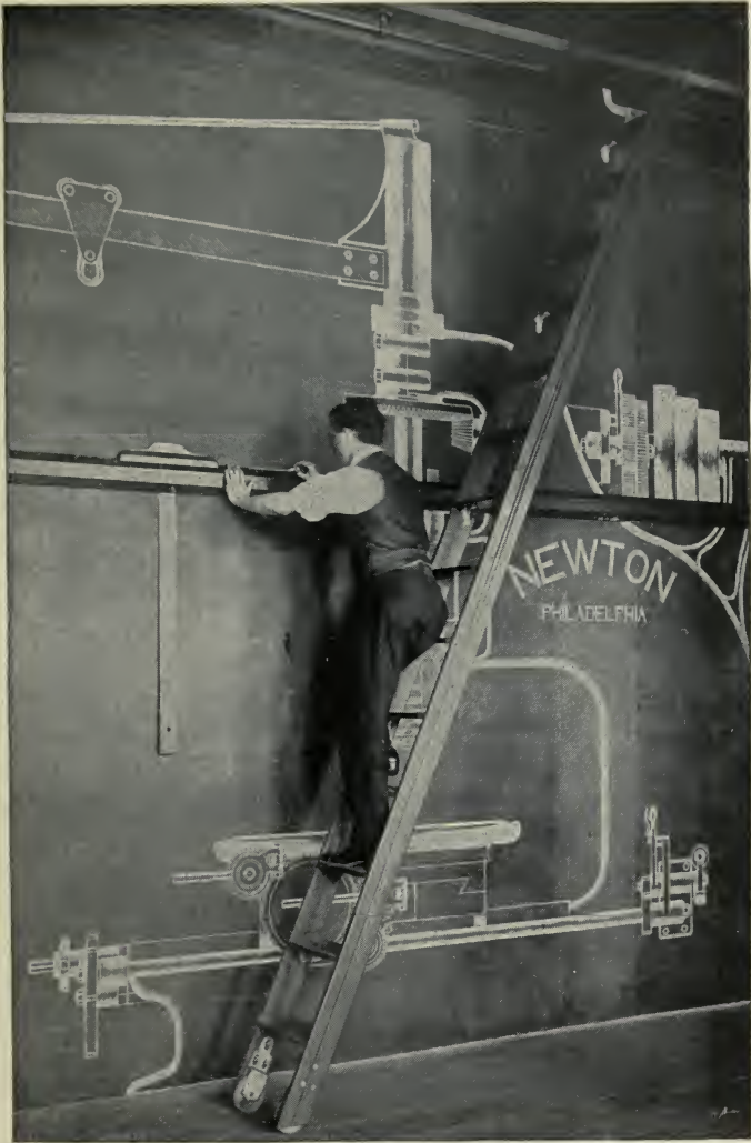
Plate II: Life size drawings of machines bring out the niceties of design in the drafting room of the Newton Machine Tool Works. A blackboard drawing outfit does the trick (See Chapter V)
