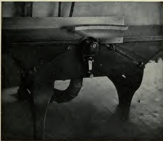
Plate X (below) and XI (above): Two devices which help reduce the accident risk. A belt shield at the Sherwin-Williams Company's plant, and (below) a planer guard at the General Electric Company's works (See chapter XI)
