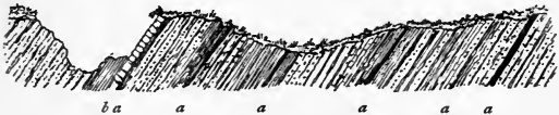
FIG. 20.—Section of inclined Carboniferous rocks, Joppa Quarry, near Edinburgh. a , coal seams; b , limestone with marine organisms. The dotted bands are sandstones, the shaded are shales and clays.
