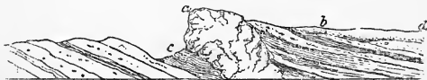
FIG. 35.—Geological section showing how a prominent feature at the surface may be caused by the outcrop of a hard rock ( a ) intercalated among softer strata.
