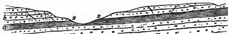
FIG. 22.—Section of a valley showing the outcrop of a junction of sandstone and shale marked by a line of springs, s, s .
