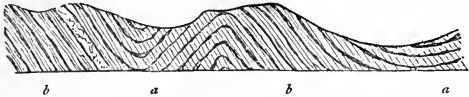
FIG. 47.—Cleavage of curved strata, coinciding with the stratification at b\ b , but at a right angle to it at a .
