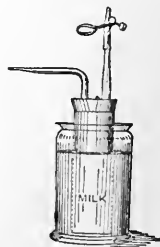
Fig. 13. — Porous Cell for the Filtration of Milk.
