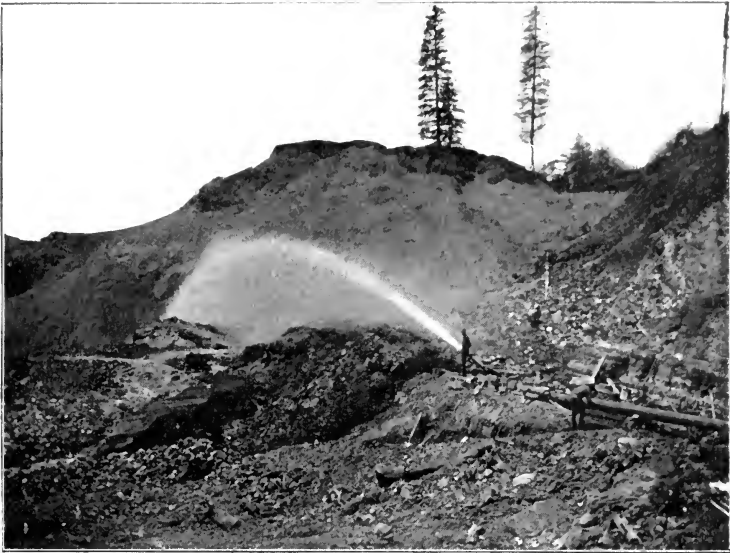
Mausard Collier Eng. Co. HYDRAULIC MINING IN CALIFORNIA. Photo. by Loyal L. Wirt. A "Monitor" at work.
