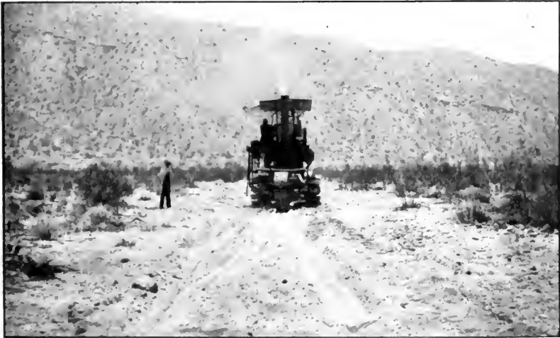
CATERPILLAR TRACTION ENGINE HAULING MATERIALS OVER THE DESERT
