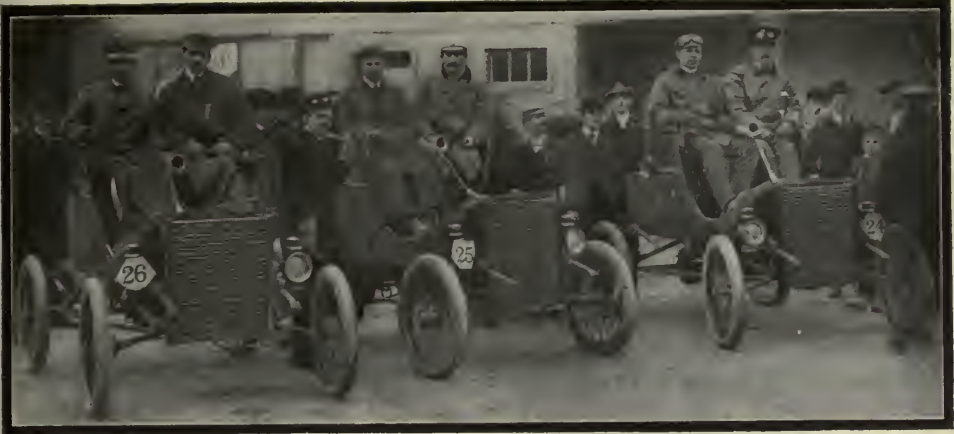
Three "White" Steam Carriages which ran in the gasoline class, and by reason of the Condensers, made the 100 miles without a stop in the "100-mile Endurance Contest" of the Automobile Club on Decoration Day.
