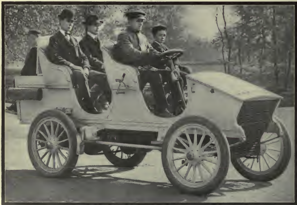
New Model "White" Steam Touring Car. The inventor, W. T. White; wheel, 20 H. P.; speed, 60 miles per hour; fastest long-distance auto ever built. This car has a "condenser"; it shows no exhaust, makes no more noise than a bicycle, and Mr. White ran the machine 200 miles without stop. ®
