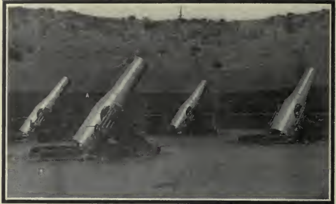
A battery of modern 12inch breech-loading mortars of our coast defense, similar to those at Corregidor.
