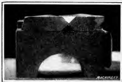
Fig. 2. Work Beveled from Both Sides
