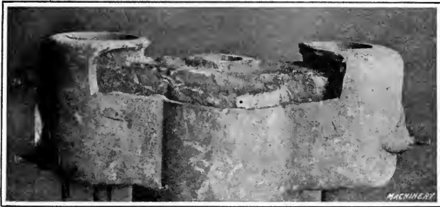
Fig. 34. Dome welded in Place
