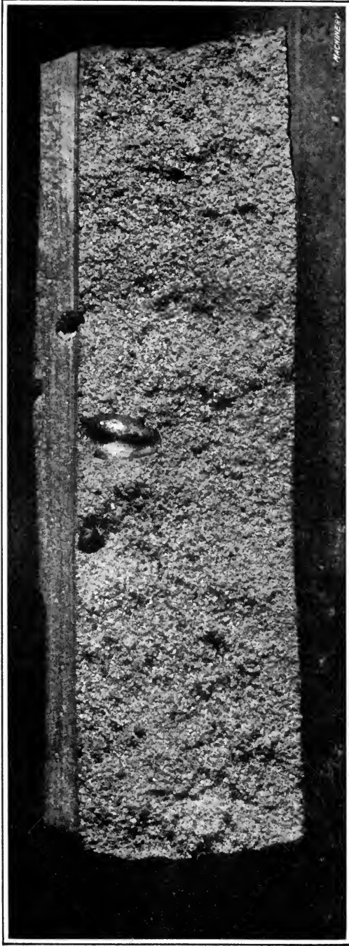
Fig. 2. Section of Cast-iron Weld broken at Right Angles to Line of Weld and magnified about Three Times. Note Uniformity in Grain of Iron
