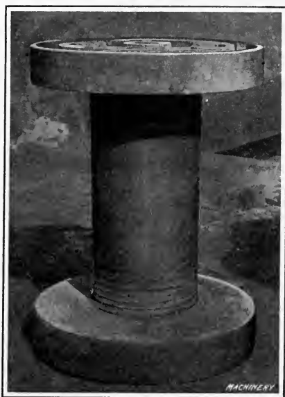
Fig. 9. Drum shown in Fig. 7 finished
