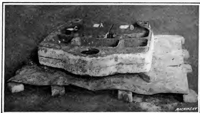
Fig. 39. Heating Boiler Casting showing Arrangement for Preheating
