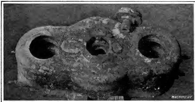
Fig. 35. Jacket welded in Place
