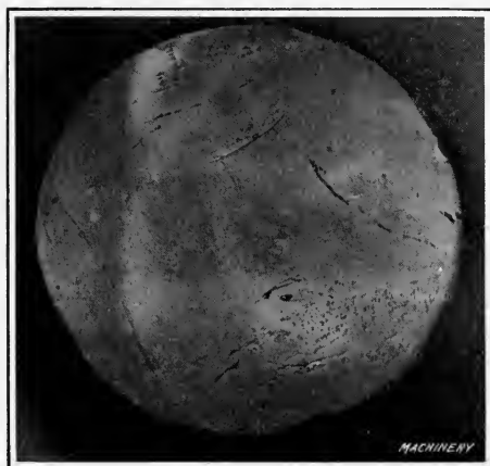
Fig. 3. Section of Defective Weld in Steel Bar
