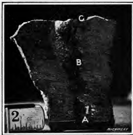
Fig. 4. Weld in Cast Iron beveled from One Side. Bottom of Weld
