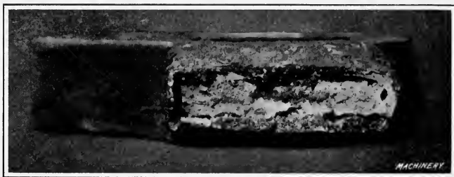
Fig. 4. Malleable Iron improperly welded
