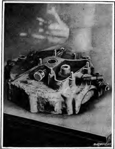
Fig. 12. Same Crankcase as shown in Fig. 10 — Finished Weld on Outside
