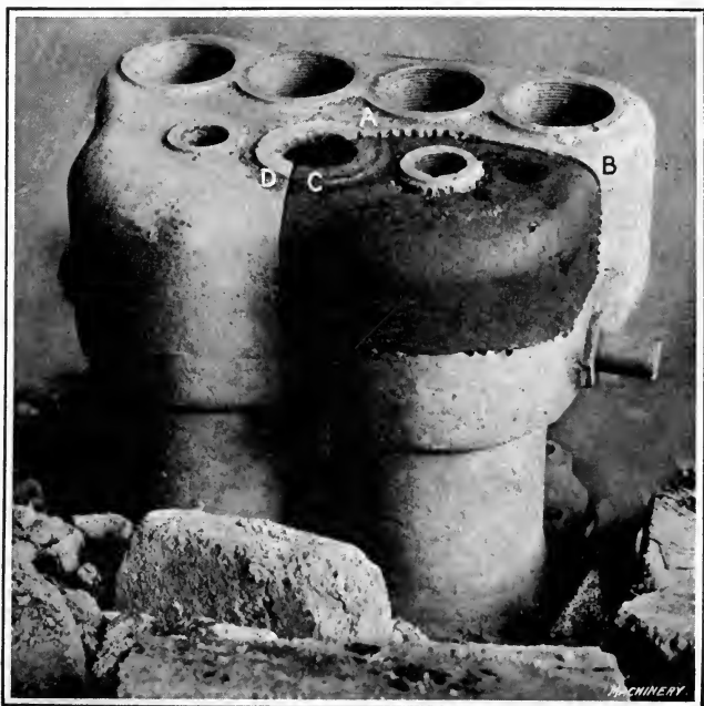
Fig. 25. Cylinder shown in Fig. 23 with Piece of Jacket set in Place ready for Welding
