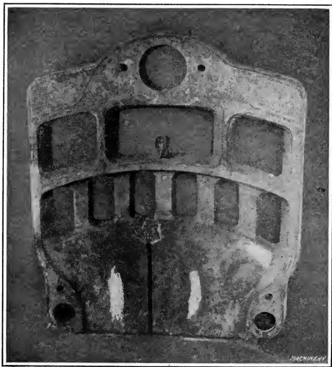
Fig. 38. Heating Boiler Casting in which Weld is finished
