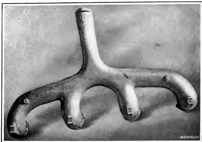
Fig. 8. Aluminum Inlet Manifold — Repairs Completed
