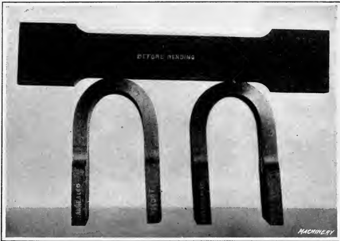
Fig. 1. Test Specimens showing Ductility of Welded Joint
