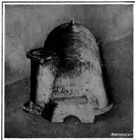
Fig. 27. Lower Half of Crankcase shown in Fig. 25, as repaired
