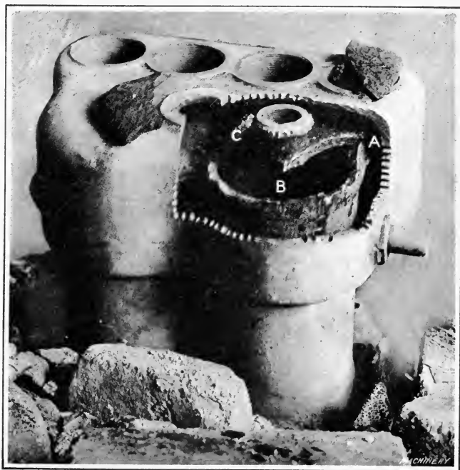
Fig. 23. Automobile Cylinder with Dome broken and Jacket cut away in Order to Reach Broken Portions
