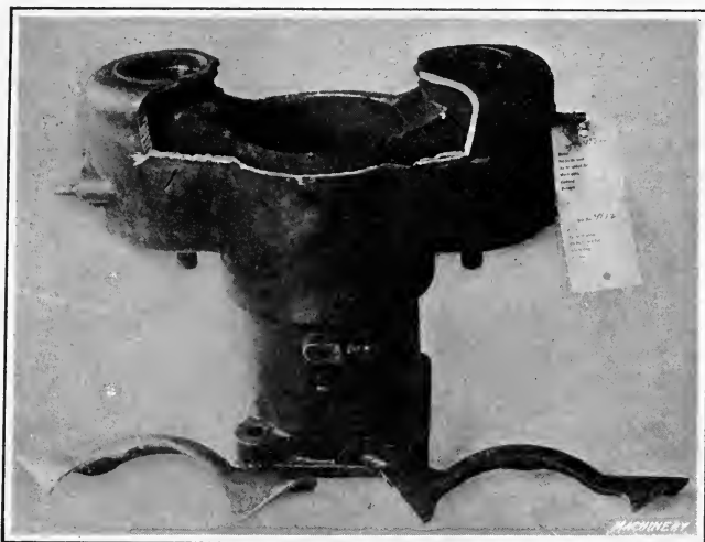
Fig. 31. Cylinder badly damaged and Jacket cut away to Enable Welding to be done
