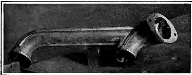
Fig. 8. Completed Weld of Manifold shown in Fig. 7
