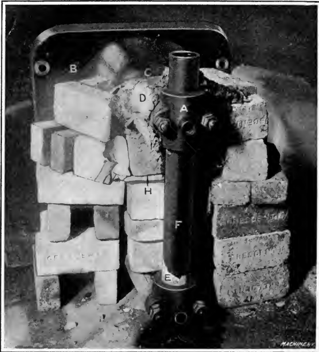
Fig. 49. Duplex Pump Base showing Method of Lining up Bearings and Saving Babbitt
