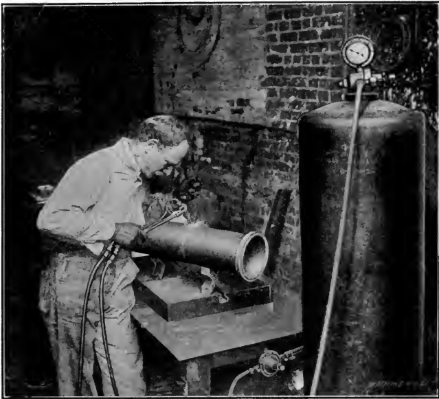
Fig. 1. Welding together the Parts of a Drawn Steel Retort. The Operator feeds the Joint with a Special Grade of Iron Wire
