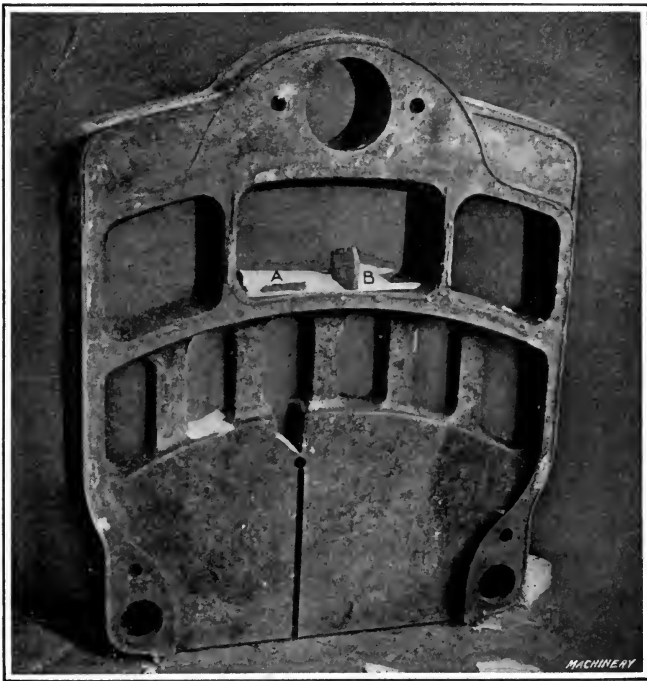
Fig. 37. Heating Boiler Casting prepared for Welding
