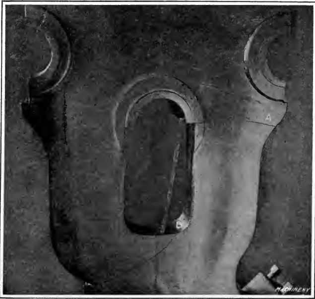
Fig. 41. Upright of Broken Press Frame
