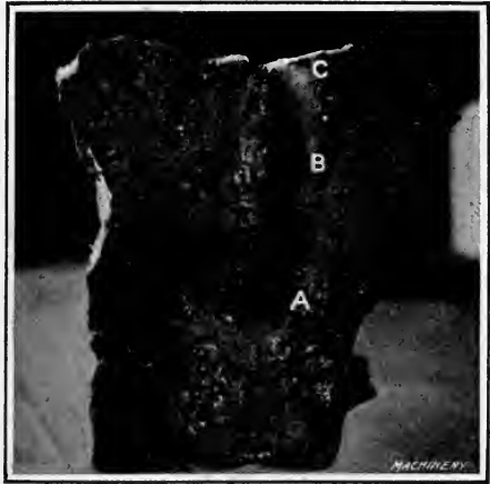
Fig. 3. Weld in Cast Iron beveled from One Side. Top of Weld
