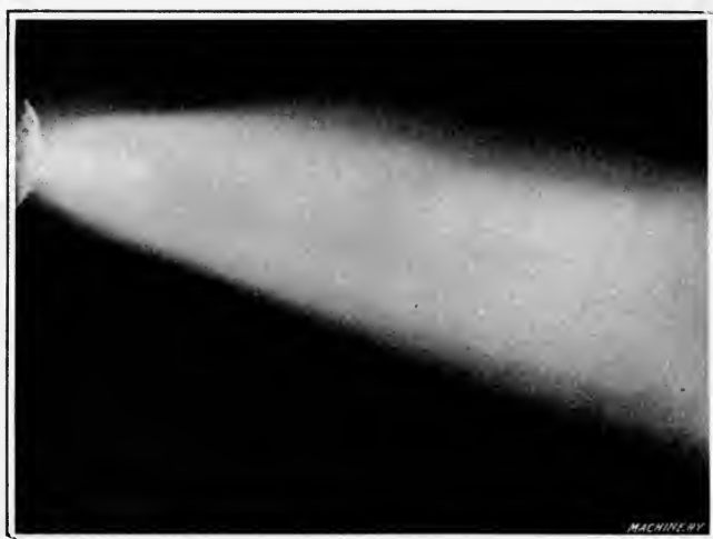
Fig. 4. Appearance of Flame with an Excess of Oxygen
