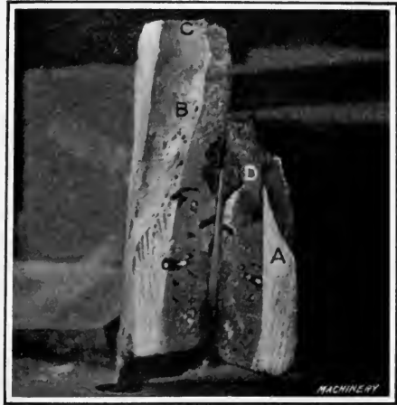
Fig. 5. Weld in Cast Iron beveled from One Side, but Broken, showing Defects
