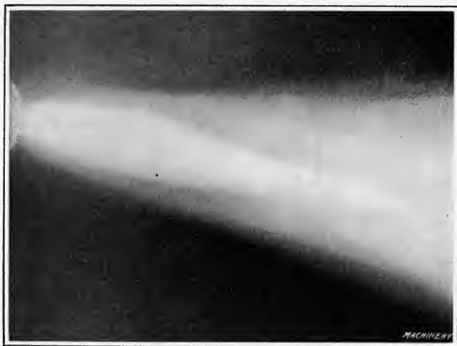
Fig. 3. Appearance of Flame with an Excess of Acetylene
