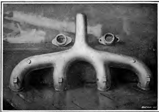
Fig. 7. Aluminum Inlet Manifold with Broken Carburetor Flange
