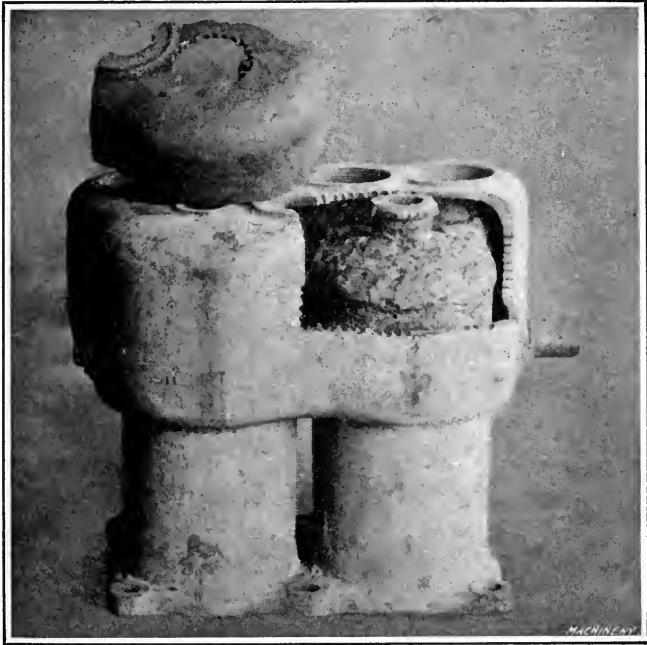
Fig. 24. Automobile Cylinder shown in Fig. 23 after Dome has been welded
