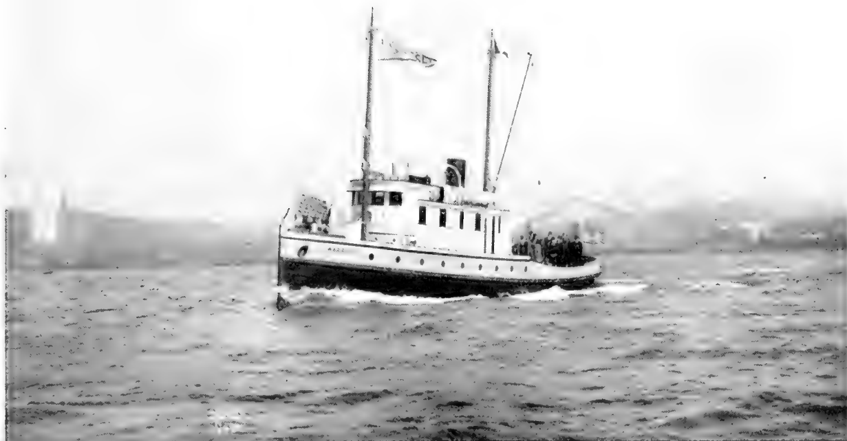
PACIFIC AMERICAN FISHERIES CANNERY TENDER WARRIOR. This is the First Cannery Tender to be Equipped With a Diesel Engine.
