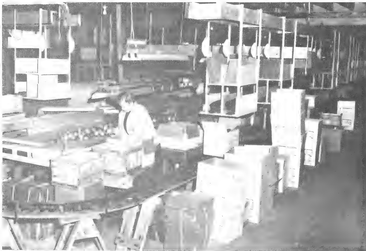
FIGURE 9.—Worker cell-packing apples from a return-flow belt. The fruit has already been sorted and sized.
