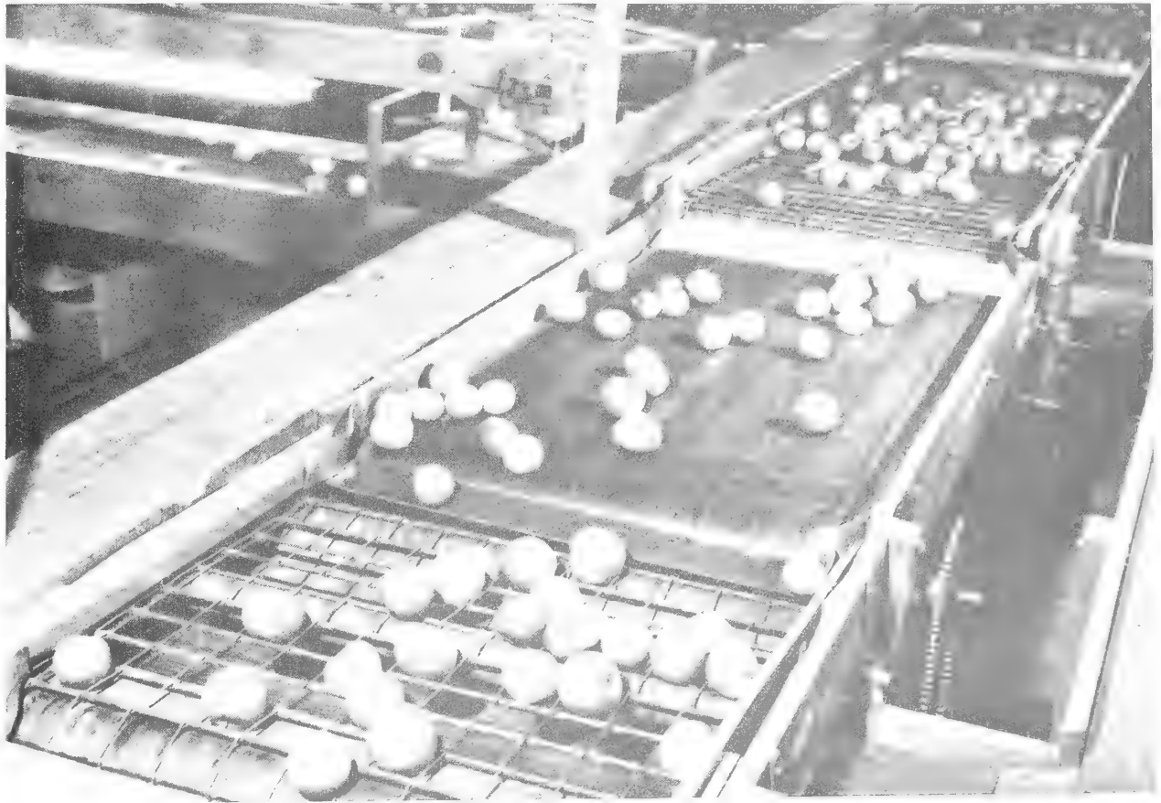
FIGURE 3.—Sizer chains and spreader belts used for apples in the Northeast area.
