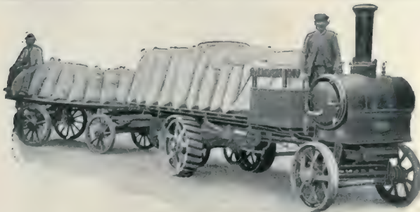
This illustration is of a Steam Wagon to carry 6 Tons and haul 4 Tons on a Trailer.
