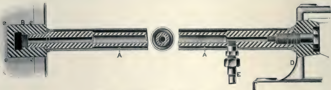
FIG. 19. STEAM-HEATED EXPANDING STAY. (Messrs. Ruston and Proctor.)
