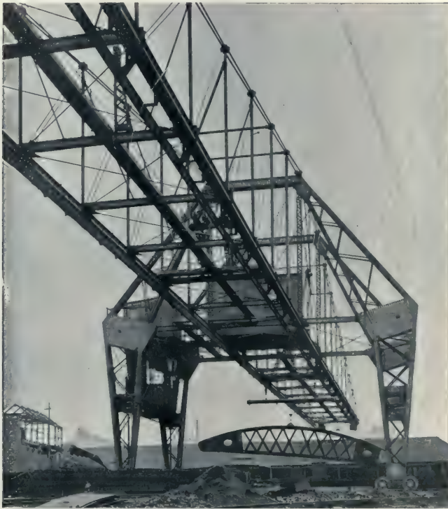
5-ton ELECTRIC TRAVELLING CANTILEVER CRANE For Stocking and Loading Material. Span, 325 ft.
