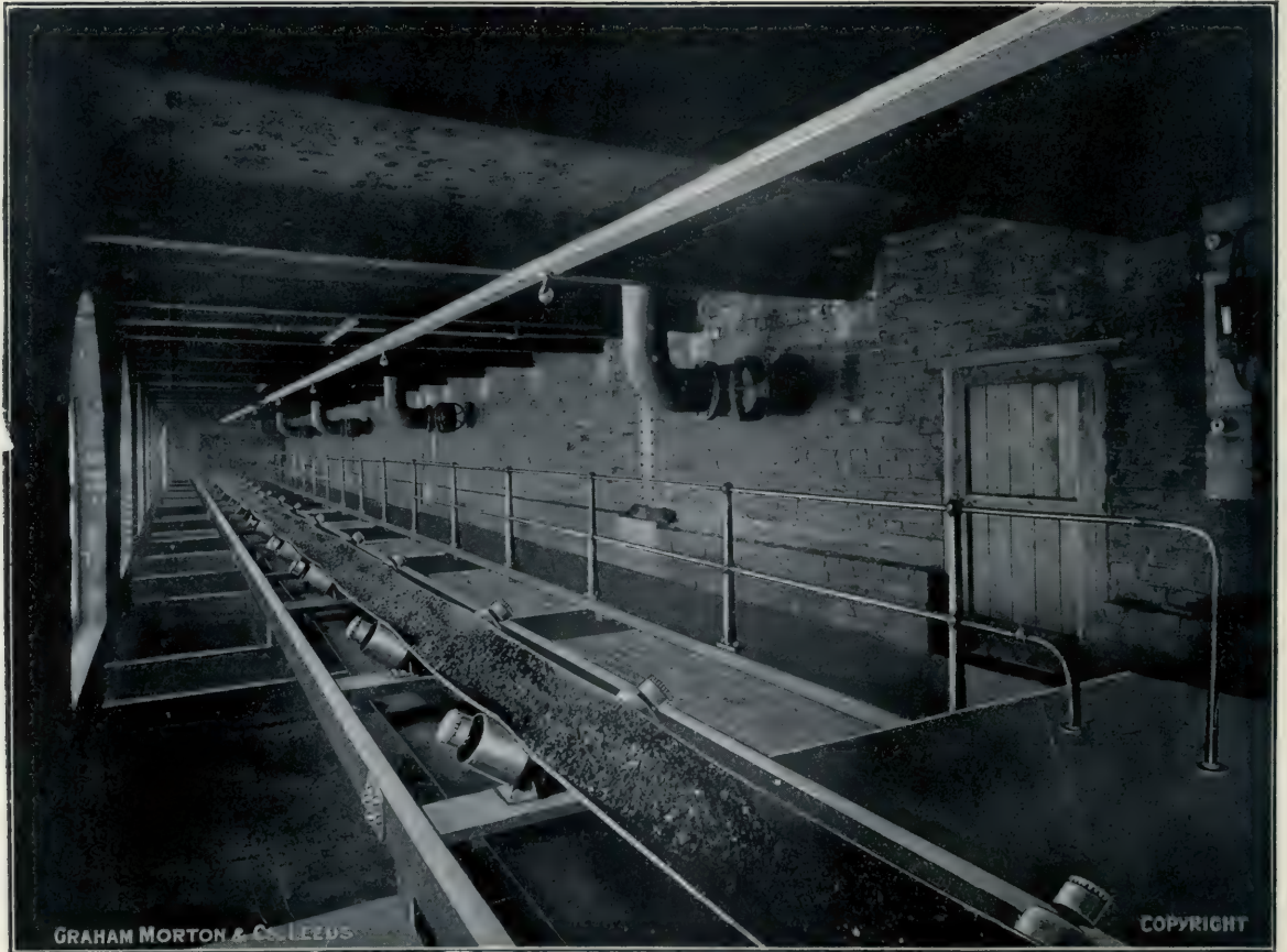
Complete Coal Conveying Plant made and erected by us for handling Coal at the rate of 50 tons per hour.
