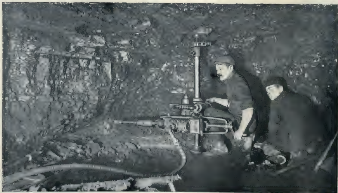
CHAMPION COAL CUTTER SET FOR HOLING OR UNDERCUTTING. READY TO START.
