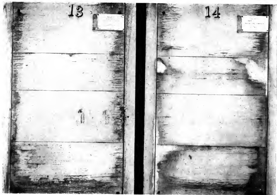
FIG. 96. Painted Panels (Impregnated with Ammonium Salts). Exposure, 18 Months.
