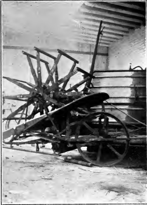
New type of Flax Harvester which pulls plant up by the roots, thus preventing infection of soil
