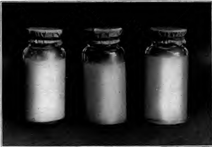
Bottles Showing Relative Permeability of Films by Amount of Whiting Formed Within
