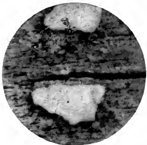
14. Test No. 13 on 1906 Fence. White Spots Show Paint Left on Wood. Balance of Paint Split and Disintegrated from Surface
