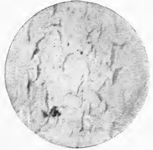
20. Test No. 8, on 1906 Fence. Surface Checking Only
