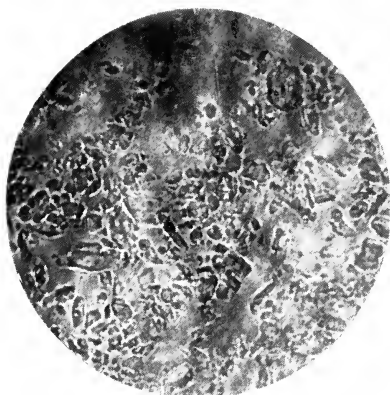
Calcium Sulphate (Gypsum)
