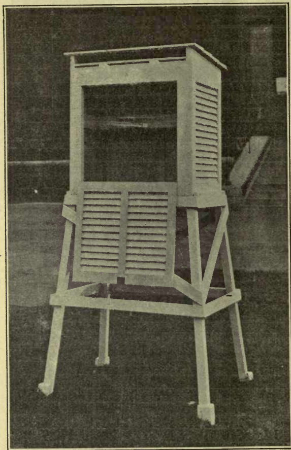
FIG. 18.—Standard type of instrument shelter used by the Weather Bureau. The shelter is always placed so that the door opens toward the north so that the sun can not shine directly on the instruments when the door is open.
