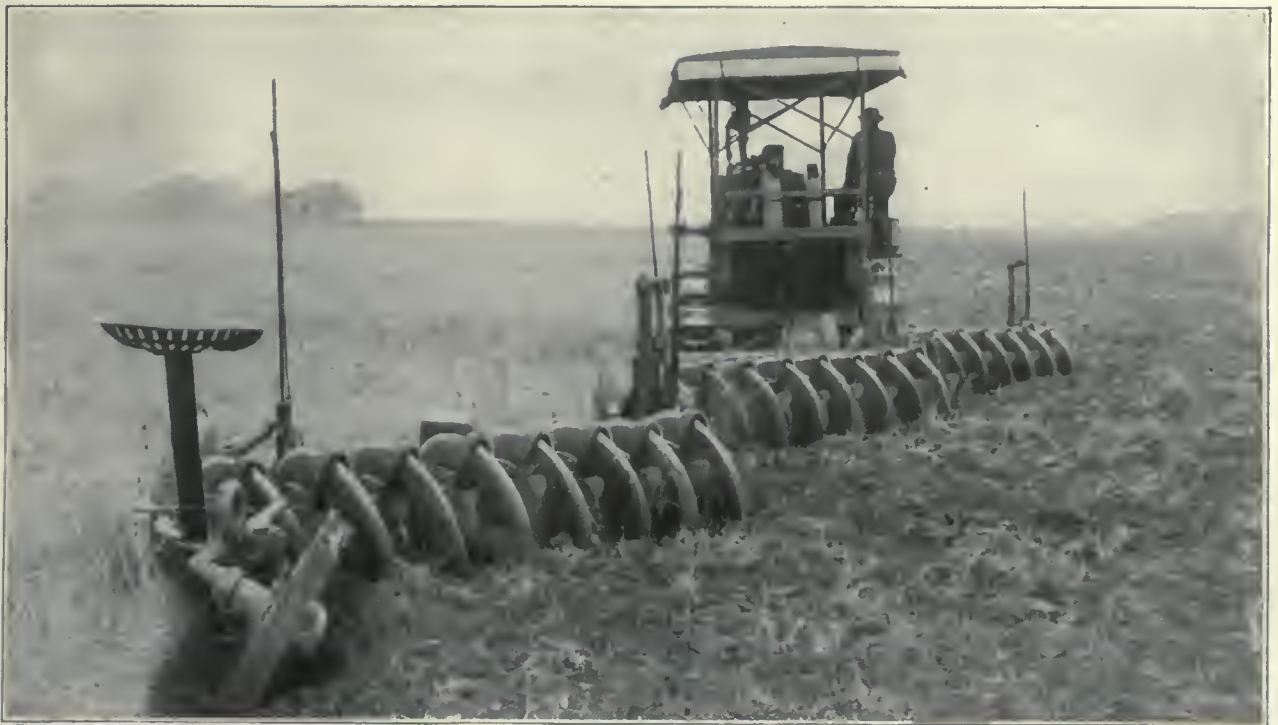
Tractor and 24 disc plows cutting a 16-foot furrow in dry sod land and covering over 4 acres per hour.
