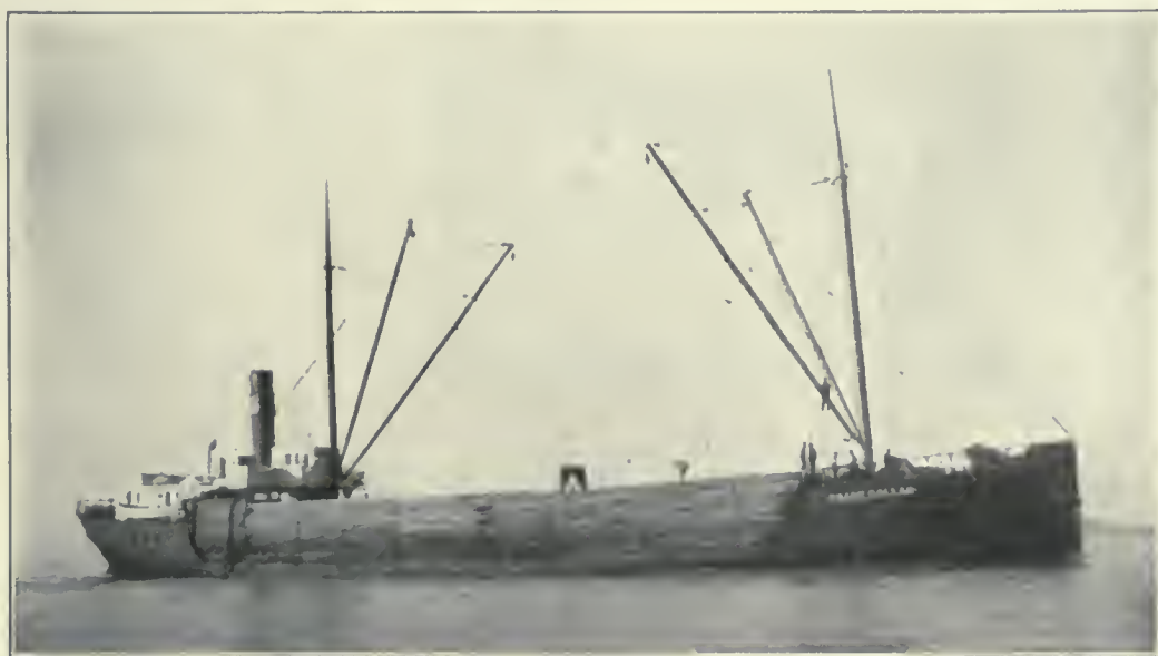
A VESSEL ESPECIALLY DESIGNED FOR TIMBER CARRYING. NOTE THE LENGTH OF CLEAR HULL AND DECK ROOM.
