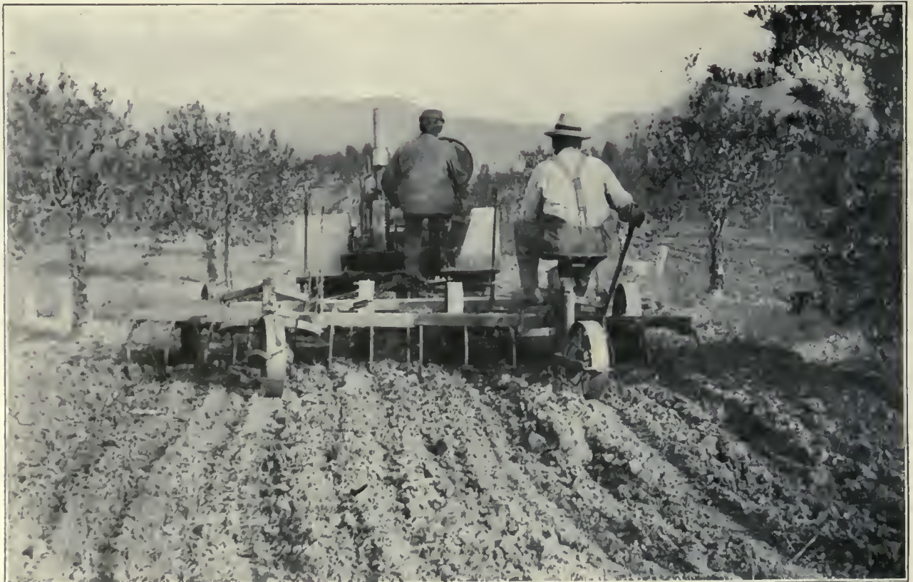
Tractor and scarifier working in an orchard to help the rapid growth of trees.
