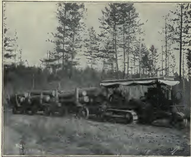
45-h. p. Caterpillar with a load of logs in woods at Newport, Wash.
