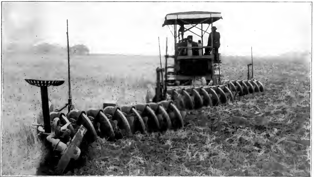
Tractor and 24 disc plows cutting a 16-foot furrow in dry sud land and covering over 4 acres per hour.
