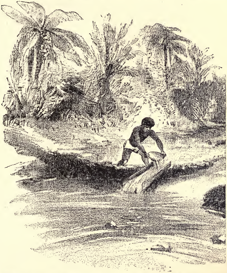
SKETCH SHOWING METHOD OF SLUICE WASHING PRACTICED AT TIPUANI.
