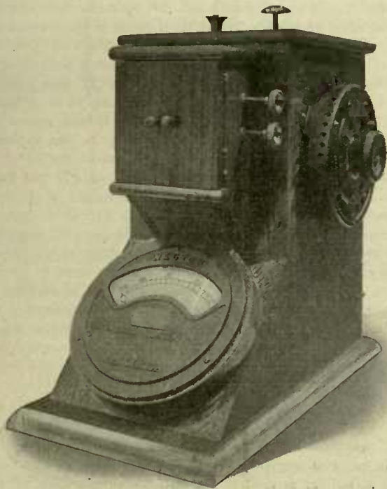
FIG. 39. VALLEY SIZE TESTER (Valley Iron Works, Appleton, Wis.)
