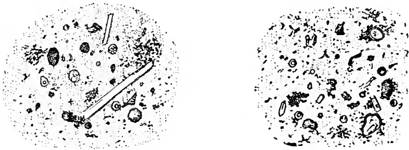
FIG. 9.—Dust of the air caught by aspiration in the meshes of gun-cotton.
