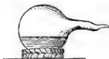
FIG. 11.—Flask used by Pasteur in his study of fermentations and of the distribution of germs in the atmosphere.
