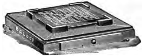
Wolffhügel's apparatus for counting colonies.
