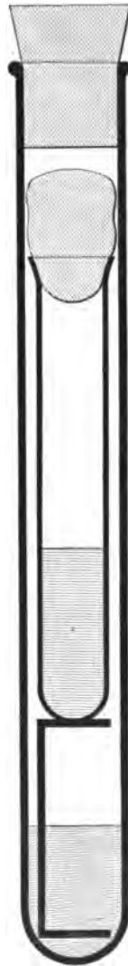
Buchner's anaerobic tube. The fluid consists of pyrogallic acid dissolved in 10 per cent. soda solution. By Wilson's method the tubes are charged with pieces of caustic potash covered with pyrogallic acid.
