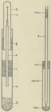
FIG. 146.—McJunkin's tube for collecting blood for cultures.
