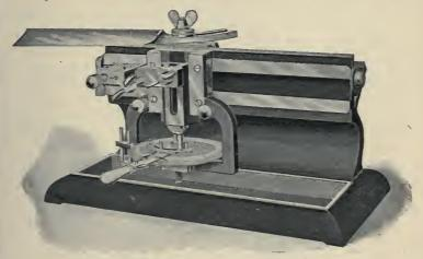
Fig. 3.—Large laboratory microtome (Bausch & Lomb).
