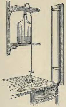
Fig. 1.—Freezing microtome.
