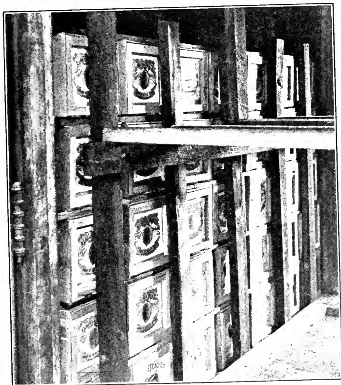
PLATE XXXI. — LOADING IN THE CAR. Top , bushel baskets properly stacked; bottom , Georgia carriers braced to prevent movement of packages in transit.
