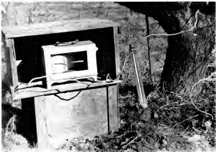
Fig. 10.—Soil thermograph and thermometer used in determining temperatures suitable for volatilization of PDB crystals.
