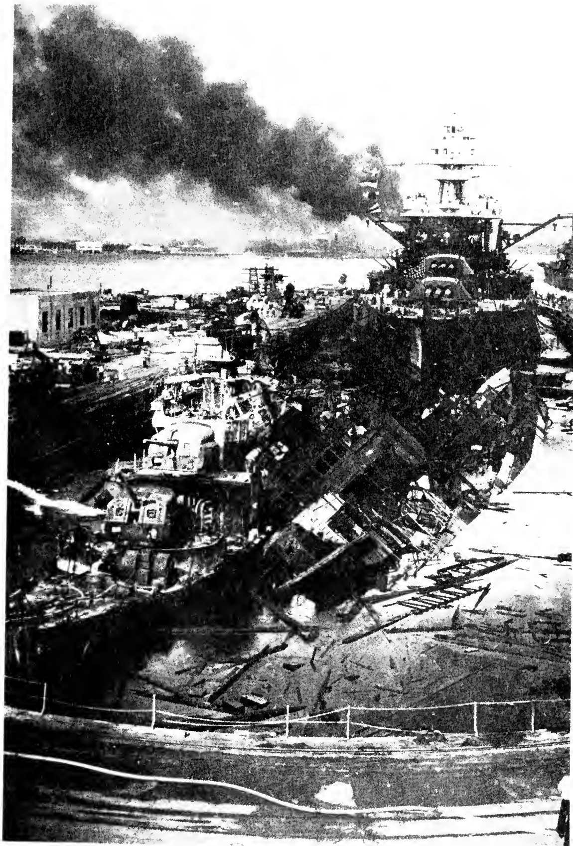
U. S. S. Downes and Cassin —The jumbled mass of wreckage in the foreground of drydock No. 1 are the U. S. destroyers, Downes (left) and Cassin (right). The battleship in the rear is the U. S. S. Pennsylvania , 33,140-ton Flagship of the Pacific Fleet, which suffered relatively light damage during the Japanese attack. The Pennsylvania was repaired shortly after the attack. Main and auxiliary machinery fittings of the Downes and Cassin are being transferred to new hulls.
