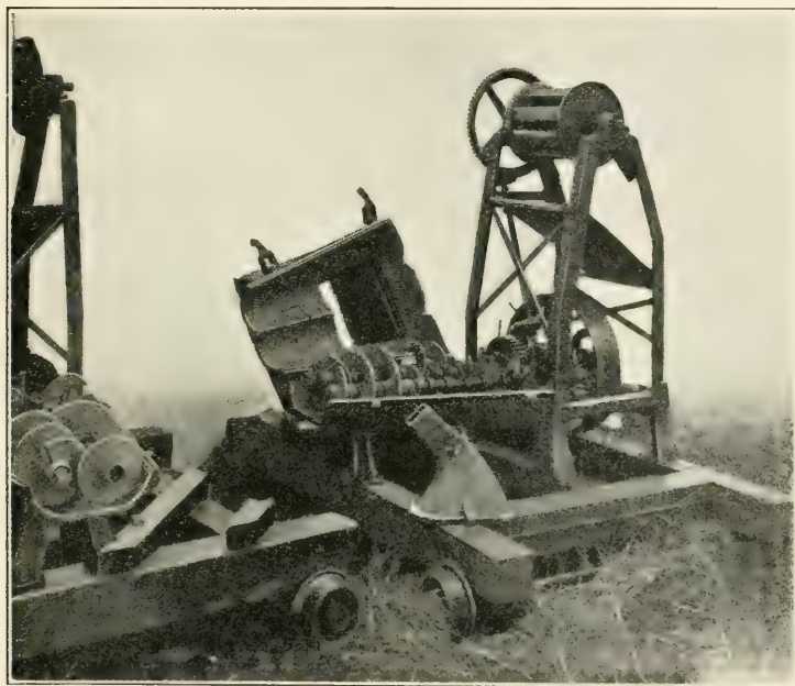
FIG. 30.—Åkerman's Peat Machine, showing Internal Arrangement.
