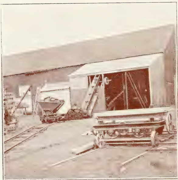
FIG. 41.—View showing Patent Lifting Bogie ; also wet Peat lying ready to go on to Elevator to Squeezer.
