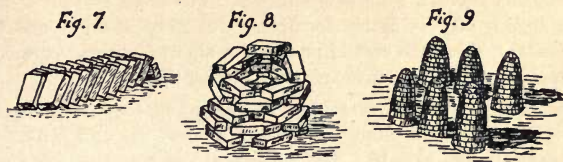
Peat Bricks turned, raised and piled in heaps for drying, Sparkaer, Denmark.
