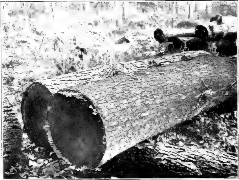
Fig. 32 WHITE OAK AND PINE LOGS ATTACKED BY FUNGI. The White Oak logs in foreground attacked by 3 different species of fungi. Cut about 8 months before photographing. The value has depreciated with exposure and fungous attack.
