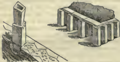
[Flues to the Floors and Walls.— From Cameron.] [Specimen of Hollow Pavement.— From Cameron.]
