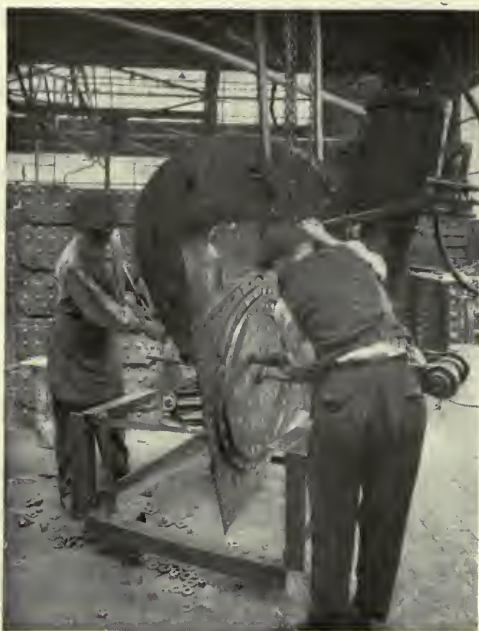
Riveting Base Ring and Base Plate, 240 mm. Trench Mortar.
