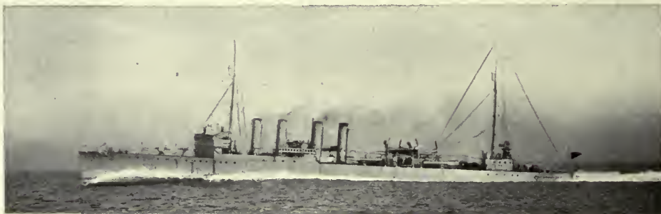
U. S. S. "Cole," on trial at sea, maintaining a speed of 41.1 Knots between 14-Fathom Bank and Brandywine Shoals Light.
