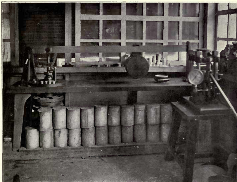
Fig. 2. Hydraulic briquetting machine for testing road materials.
