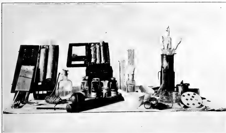
Fig. 1. Apparatus used in a field assay of water.
