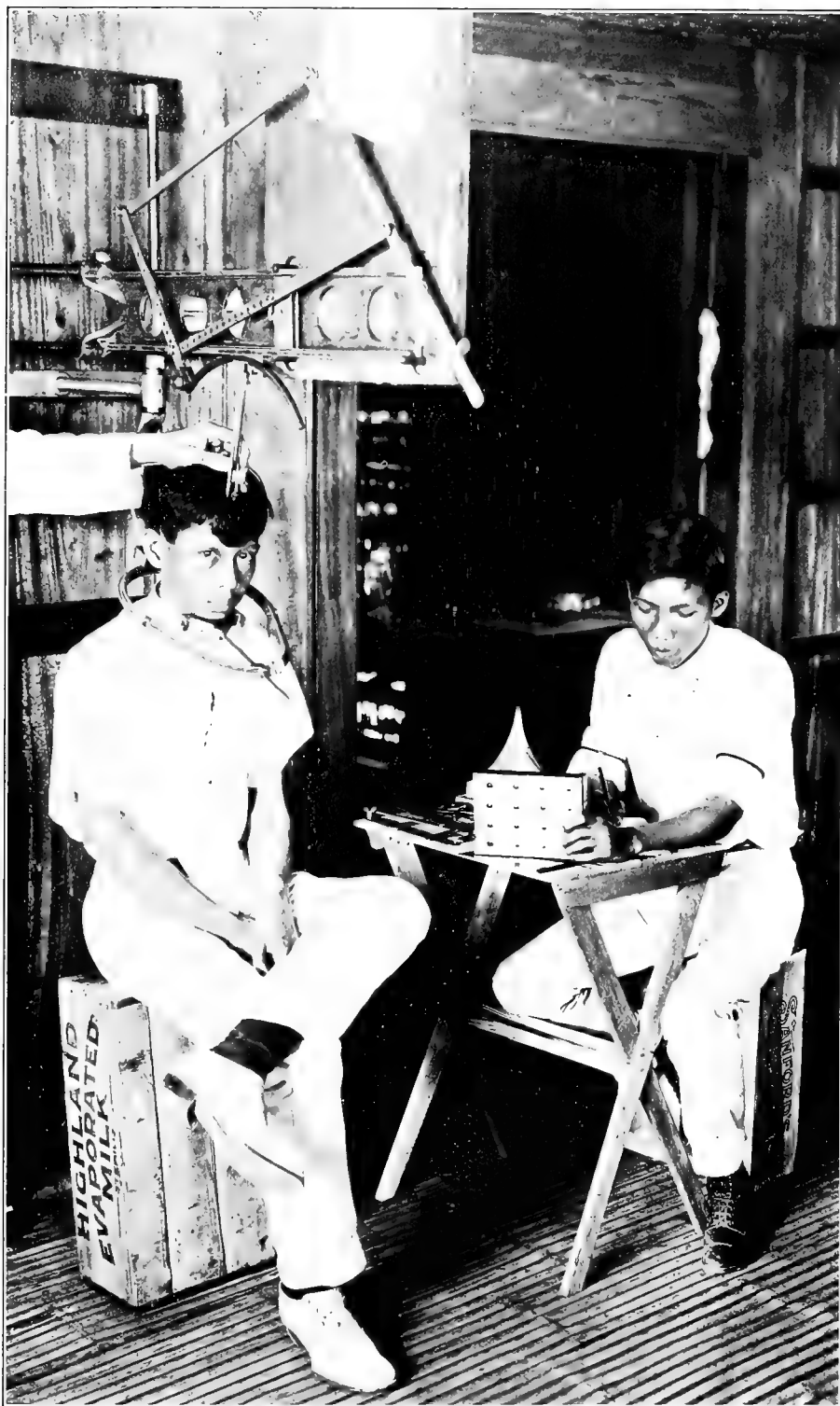
VENTRO-LATERAL VIEW OF THE CEPHALOGRAPH AT WORK AT TAYTAY, PROVINCE OF RIZAL, ISLAND OF LUZON, IN 1909.
