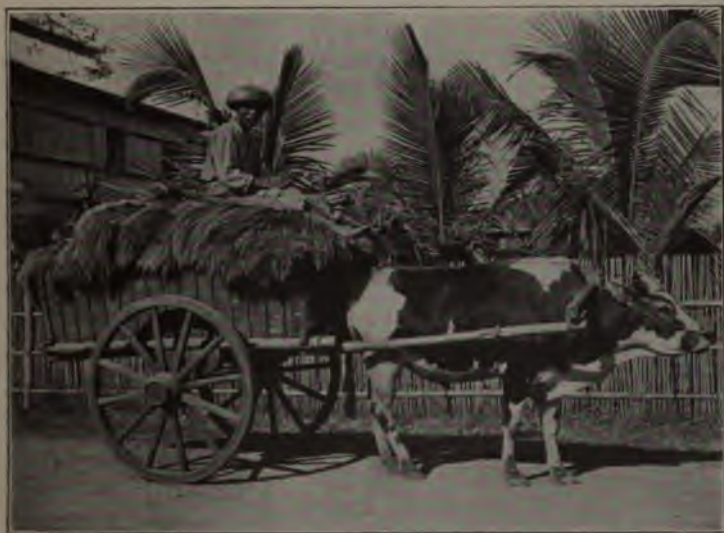
A new-style cart, with broad-tired wheels, which does not injure the roads.
