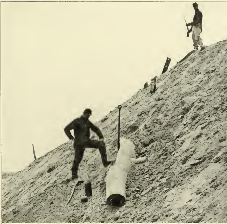
THE LARGEST CONFEDERATE GUN AT YORKTOWN—A 64-POUNDER BURST IN THE EFFORT TO REACH FEDERAL BATTERY NO. 1 IN MCLELLAN'S WORKS BEFORE THE BELEAGUERED CONFEDERATE CITY
