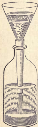
FIG. 11. made by placing in the funnel an excess of the substance to be dissolved.
