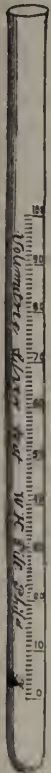
Fig. 2. which the above salts, as they increase its density, test by the hydrometer as so much silver, and we cannot tell, from its indications, how much nitrate of silver alone it contains. The older the bath, the more impure the solution, and the more unreliable this manner of testing becomes. The reason of this I have given above.
