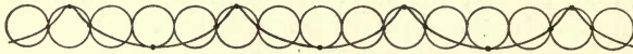
FIG. 16. The phasal difference of the particles has been increased from 45^\circ to 90^\circ . The crests of the waves thus become sharper. (After Fenneman.)
