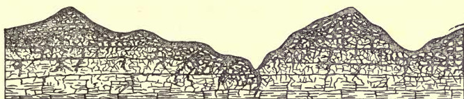
FIG. 13. Diagram showing the relation of residual soil to the underlying rock from which it is derived. (Courtesy of U. S. Geol. Surv.)
