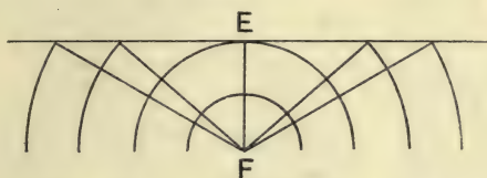
FIG. 97. Seismic focus ( F ) and epicentre ( E ) of an earthquake.
