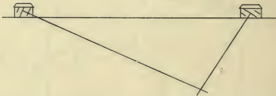
FIG. 100. Determination of depth of seismic focus.
